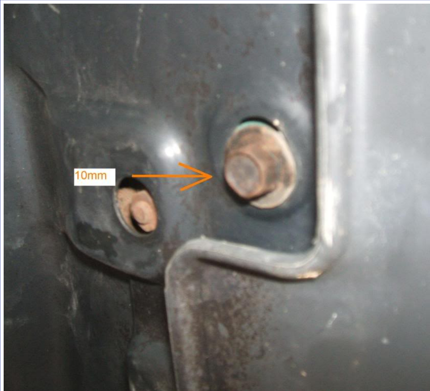
Splash shield removed.
