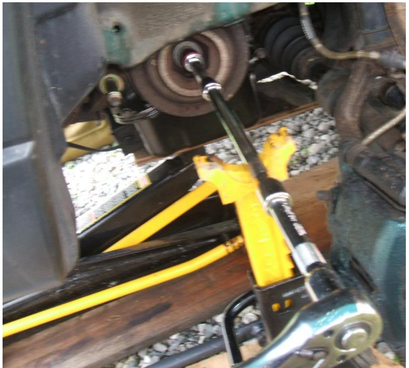
Align the white mark (red arrow) with the alignment tab (yellow arrow) on the crank shaft pulley and lo
